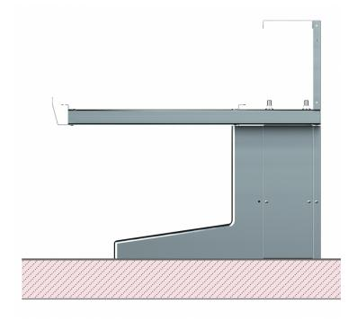
Construction - Basic structure made in galvanized iron 4mm thick. Structure for support cooking appliances in stainless steel CrNi 18/10 304 with 3 mm thick. External panels with Stainless Steel Scotch-Brite Satin polish Finish, rounded edges, chromed details. Model - Cantilever structure for professional kitchens, designed for the support of the Iperlotus 90 line. Maintenance - All serviceable parts are accessible by the easy removal of front external panels.
