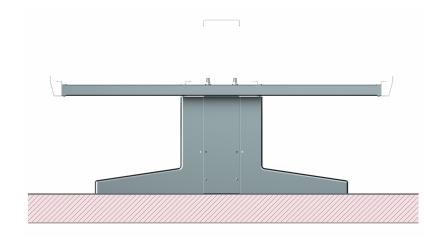
Construction - Basic structure made in galvanized iron 4mm thick. Structure for support cooking appliances in stainless steel CrNi 18/10 304 with 3 mm thick. External panels with Stainless Steel Scotch-Brite Satin polish Finish, rounded edges, chromed details. Model - Cantilever structure for professional kitchens, designed for the support of the Superlotus 70 line. Maintenance - All serviceable parts are accessible by the easy removal of front external panels.
