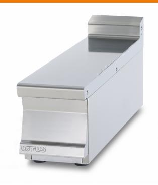
Construction - Fabricated using CrNi 18/10 AISI 304 grade Stainless Steel Scotch-Brite Satin polish Finish, incorporating 2 mm thick worktop, rounded edges, chromed details and rear splash back. Model -Professional worktop with or without drawer . Fittings - Appliance is supplied with steel or plastic tanks, h 15cm. Adjustable feet.
