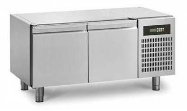
Construction - Fabricated using CrNi 18/10 AISI 304 grade Stainless Steel Scotch-Brite Satin polish Finish, rounded edges and chromed details. Model - Refrigerated stand with doors and drawers, for professional use. Condensing unit incorporated, Refrigerant Gas R290. Automatic electric defrosting. Insulation with foam without CFC and HCFC. Fittings -Appliance is supplied with adjustable feet.
